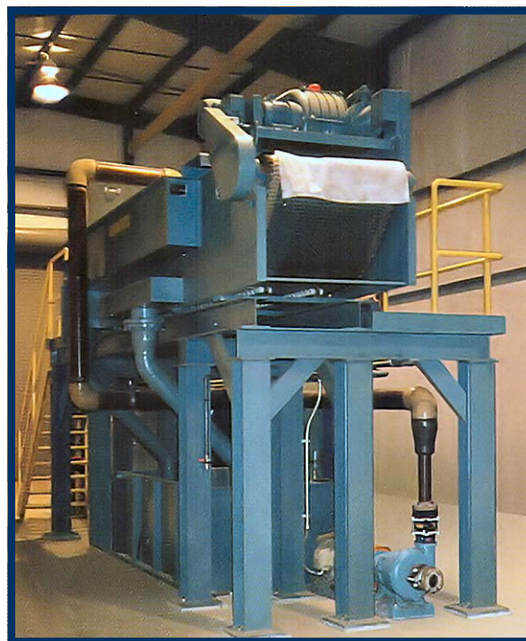
F-750 shown at a customer's plant filtering contaminated water from a mill hotwell
