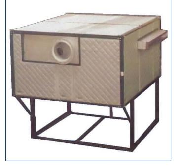
**Horizontal Header Support Table** with four (4) sets of 6" (152 mm) diameter, 30° "V" headers with adjustable slots, entry and exit EDPM-coated header protection rolls (not shown), and air distribution box. This unit is used to dry steel strip after cleaning at 968 ft./min. (295 m/min.), 49" (1245 mm) strip width.
