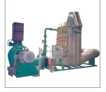
**Strip Drying System** with a steam heater on a pushpull pickle line. This system is designed to dry 72" (1830 mm) wide strip at speeds of up to 500 ft./ min. (152 m/min.).
