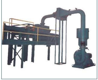
Vertical Header Support Structure with three (3) sets of 6" (152mm) diameter, 15° "V" headers with adjustable slots, entry and exit EPDMcoated header protection rolls, and air distribution box. This unit is used to dry steel strip after quenching at 600 ft./min. (182 m/ min.), 49" (1245mm) strip width.
