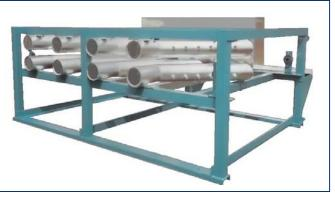
**Strip Drying System** with an indirect fired gas heater located after chemical treatment. This system is designed to dry 72" (1830 mm) wide strip at line speeds of up to 600 ft./min. (182 m/min.).
